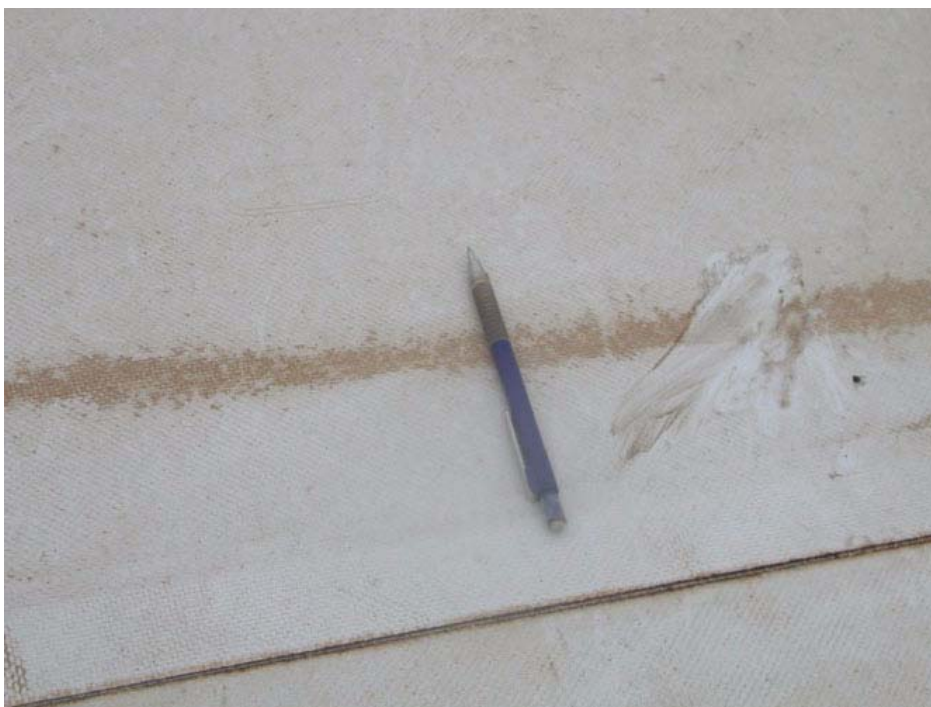
Figure 7 – soiling in lines on surface of weldable PVDF/PVC-coated polyester
