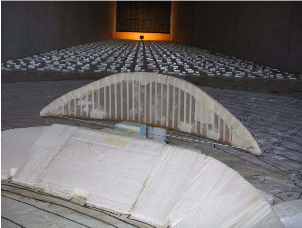
Figure 7: The 1:300 scale impermeable model of the LED screen for the 2006 Asian Games, Doha connected to the force balance.
