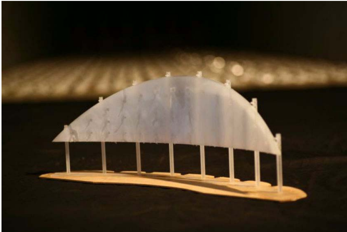
Figure 10: The 1:300 scale pressure-tapped impermeable model of the LED screen for the 2006 Asian Games, Doha.
