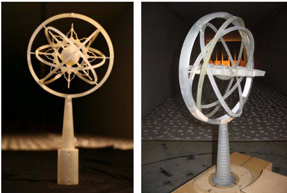
Figure 5: The 1:50 scale model of the Cauldron for the 2006 Asian Games, Doha. Left: On the force balance before inclusion of the Khalifa Stadium section model. Top Right: Within a section of the Khalifa Stadium and using the pressure correlation technique.
