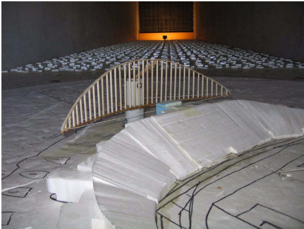
Figure 6: The 1:300 scale porous model of the LED screen for the 2006 Asian Games, Doha connected to the force balance.
