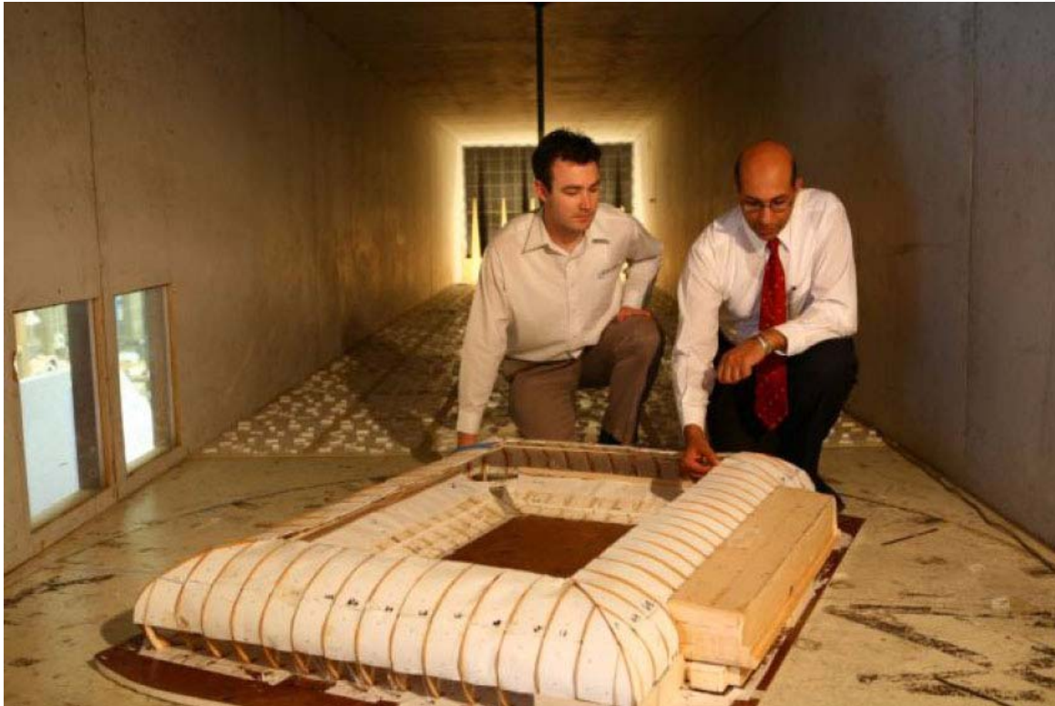
Figure 1: The 1:150 scale model of the Gold Coast Stadium in Windtech's Boundary Layer Wind Tunnel.
