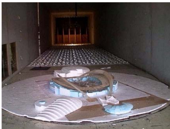
Figure 3: The 1:300 scale model (left) and a diagram showing the different patch areas (right)
