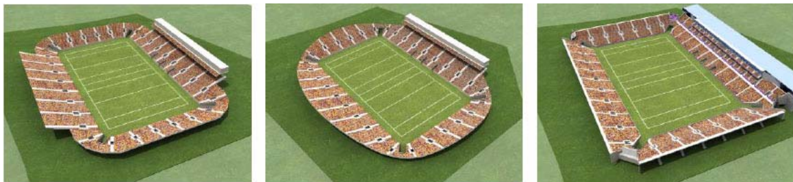
Figure 2. Some of the early seating bowl design options. The image on the right shows the option chosen.
