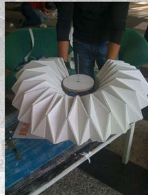
positioning of unfolded umbrella on assembly jig model
