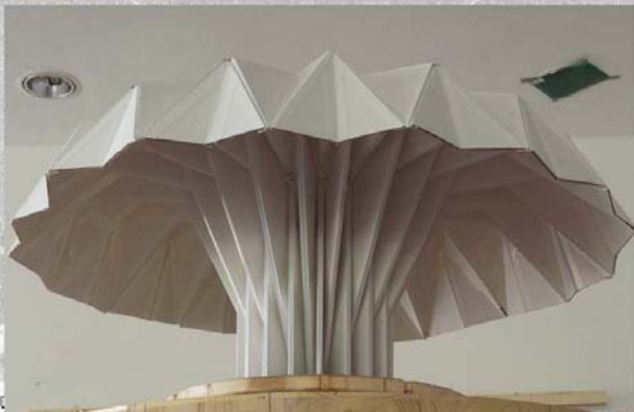
Completed 1:5 model: the entire prototype construction process was developed and confirmed here
