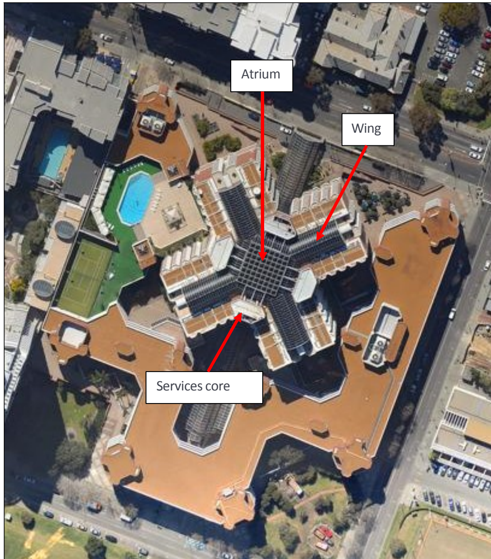
Figure 1: Roof view (source: nearmap.com)
